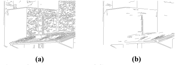
Figure 3. (a) The output of Canny edge detector and (b) morphological filtering on Fig. 1(a)
